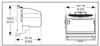
Figure 6. FP-DO-403 Mechanical Dimensions
